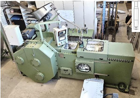
The press is designed for the necking and calibration of ammunition cases of steel or brass.
