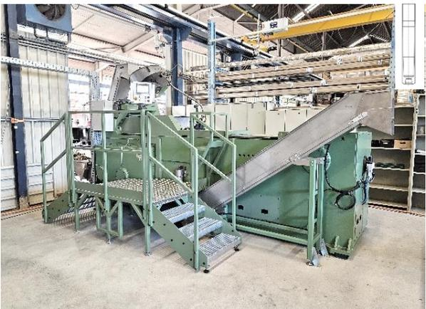
The press is designed for heading and indenting steel or brass ammunition cases.
