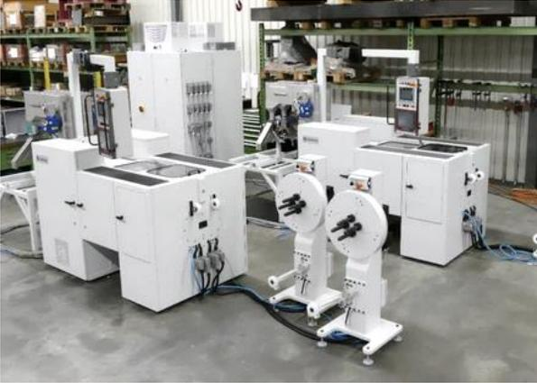
Lead core presses are suitable for forming bullet cores made of lead and tin wire
