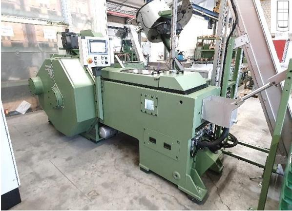
This press is designed for the drawing of ammunition cases made of steel or brass.
